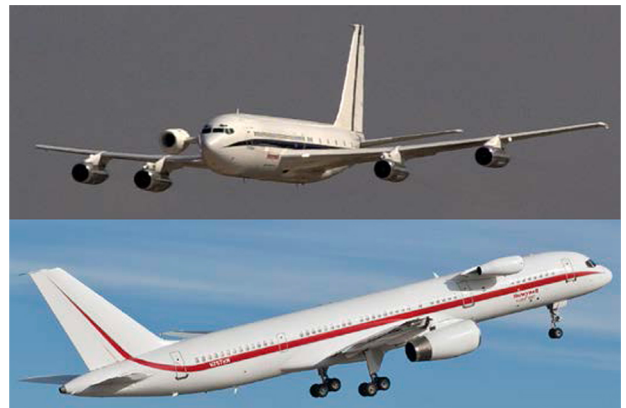
Figure 14. Honeywell's flight test vehicles for certification and endurance flights: B720 with HTF7000 installed & B757 with HTF7500 installed [Photo Credit: Eugene Cupps]
