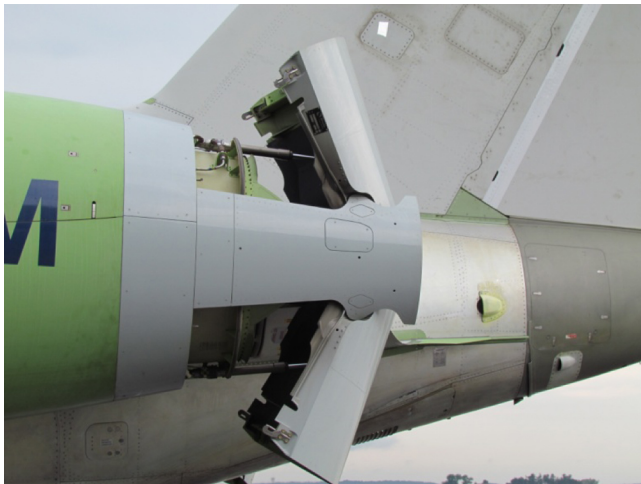
Figure 13. Installed and deployed thrust reverser for HTF7000.
